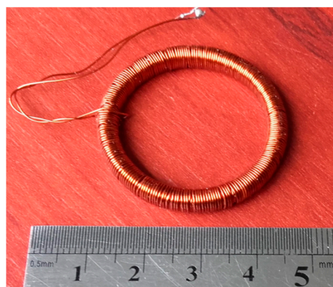
Figure 1. Typical sample used in the investigation, a ring-shaped core with a small cross-section, with 400 sensing windings, ensuring high measurement signal. Magnetization was provided with a straight magnetizing rod, which ensured a homogenous magnetizing field in the sample.
