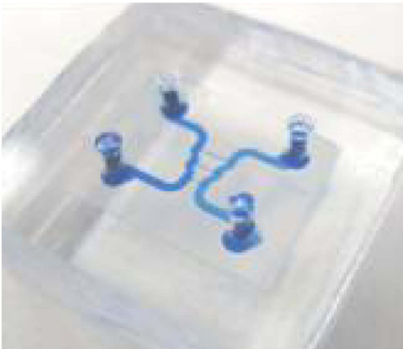
Fig. 3. A fabricated device for the linear profiles. Channels are filled with ink for visualization.
