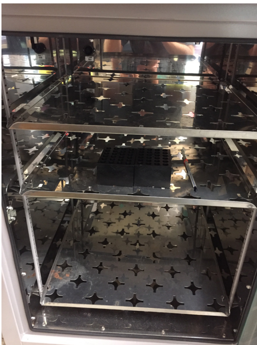
Figure 2. 40 \pm 1 °C incubator setup. Two heat blocks are stored in the incubator to regulate
