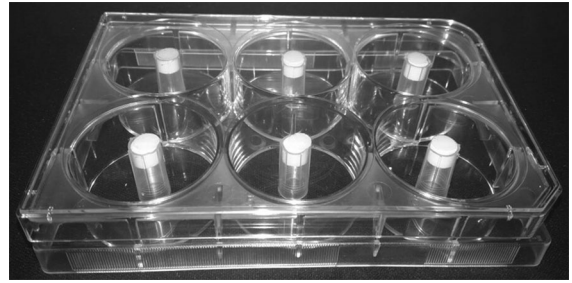
Fig. 2 Representative image of modified-6-well culture plate prepared for s-ARU method migration assay. Shortened-1 ml pipette tips were fixed in the center of each well-cover using silicone adhesive, for creating a cell-free gap in the plate
