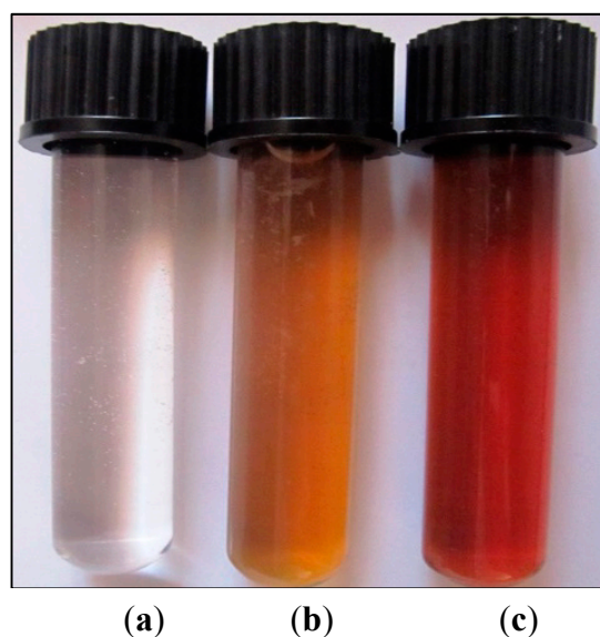
Figure 1. Visual appearance of vials containing the S. Officinalis extract and AgNO 3 solution after different reaction times: (a) AgNO 3 5 mM, (b) Aerial part extract S. officinalis , (c) AgNO 3 .
