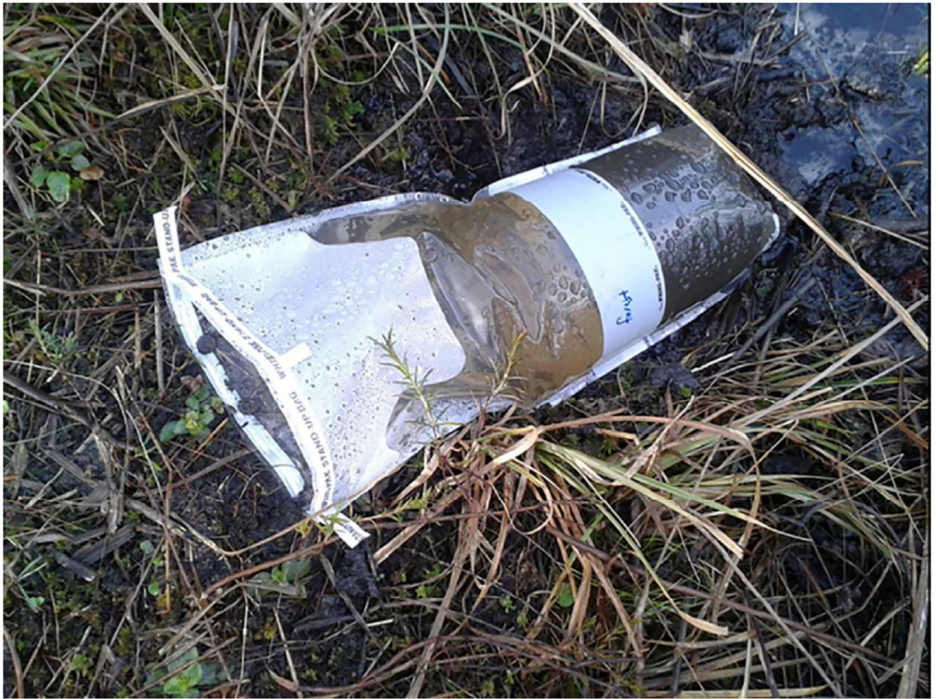
Figure 2. A storm runoff sampling bag after a storm.
