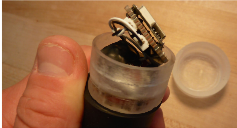
Fig. 7. Electronics outside of the housing connected to the FSR
