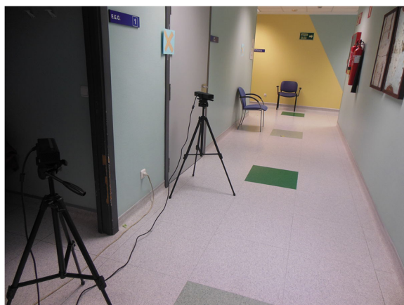
Fig. 1 Real image of the test scene. In the image you can see the two Kinect cameras and the corridor through which the patients perform the walk
