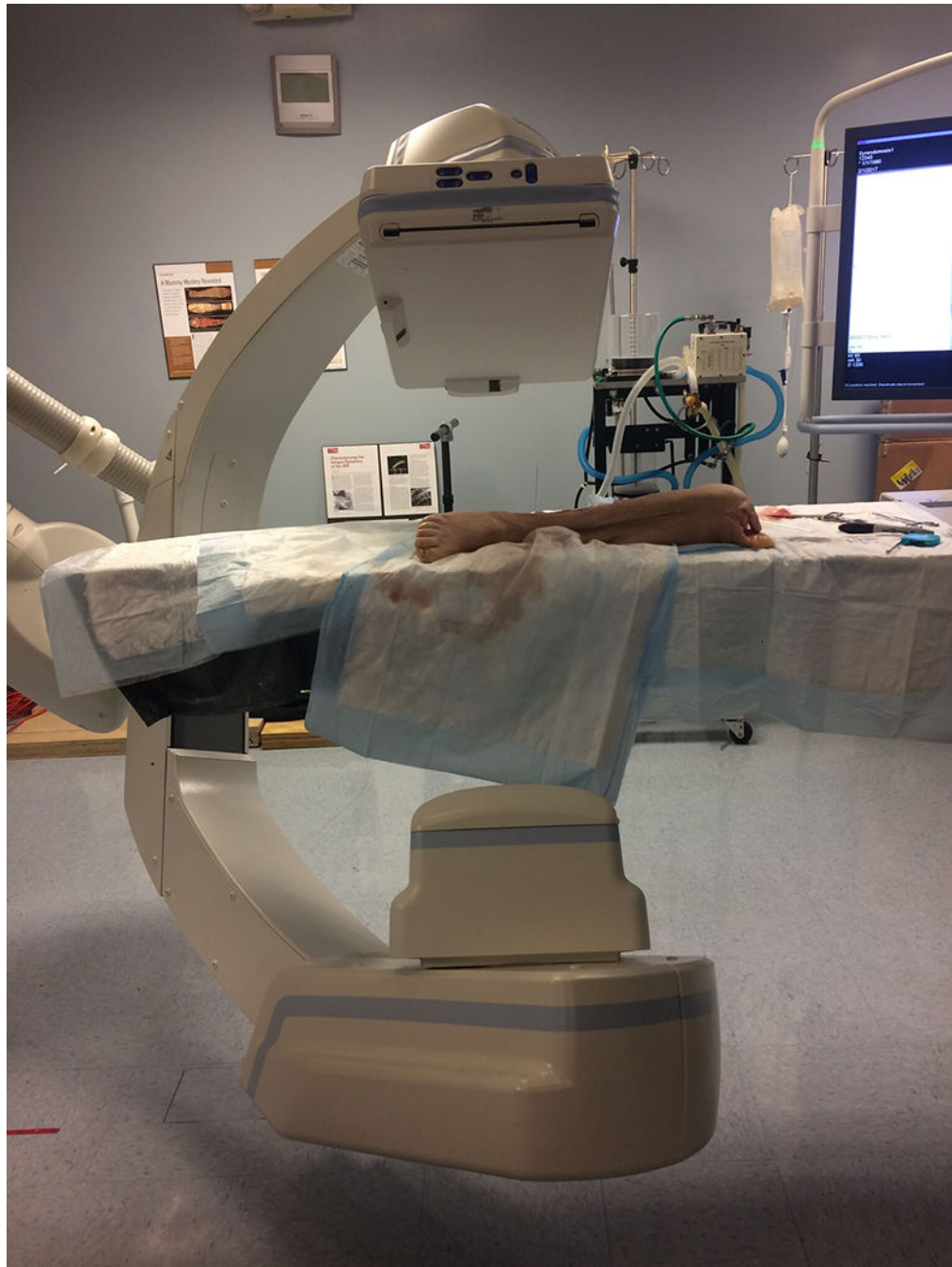
Fig 3. Image demonstrating CBCT system used to obtain axial imaging for assessment of reduction quality.
