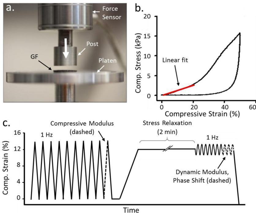
**Figure 3.** Mechanical characterization protocol of GF and GF-tissue composites. **a)** The testing apparatus was assembled to compress the GF with homemade compression platens. **b)** A typical stress-strain curve for GF displays elastic behavior between 0–14% compressive strain. **c)** The testing method designed to measure the quasi-static and viscoelastic compressive properties of GF with and without cell culture (not drawn to scale).
