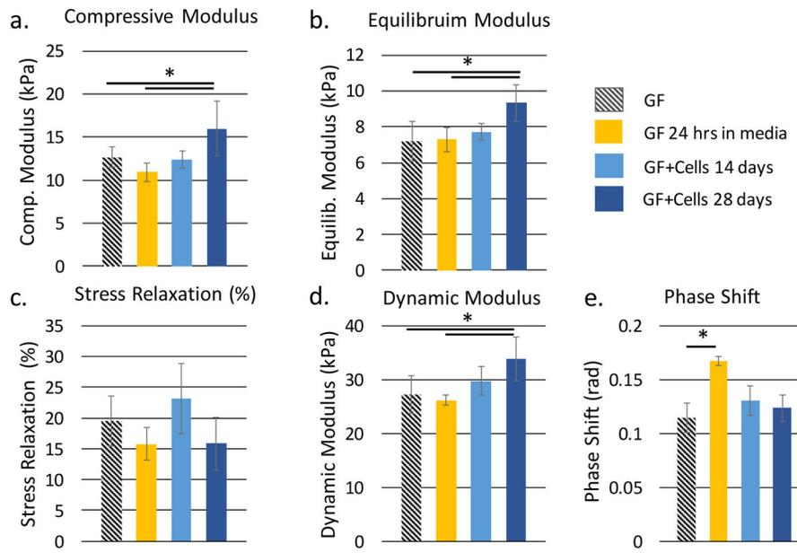
**Figure 4.** The measured quasi-static **a,b**) and viscoelastic **c–e**) properties of conditioned graphene foam (GF), graphene foam after 14 days of cell culture in chondrogenic medium (GF+C 14 days) and graphene foam after 28 days of cell culture in chondrogenic medium (GF+C 28 days).
