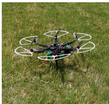
Figure 4. A prototype of the unmanned aerial vehicle (UAV)-based air monitoring system.
