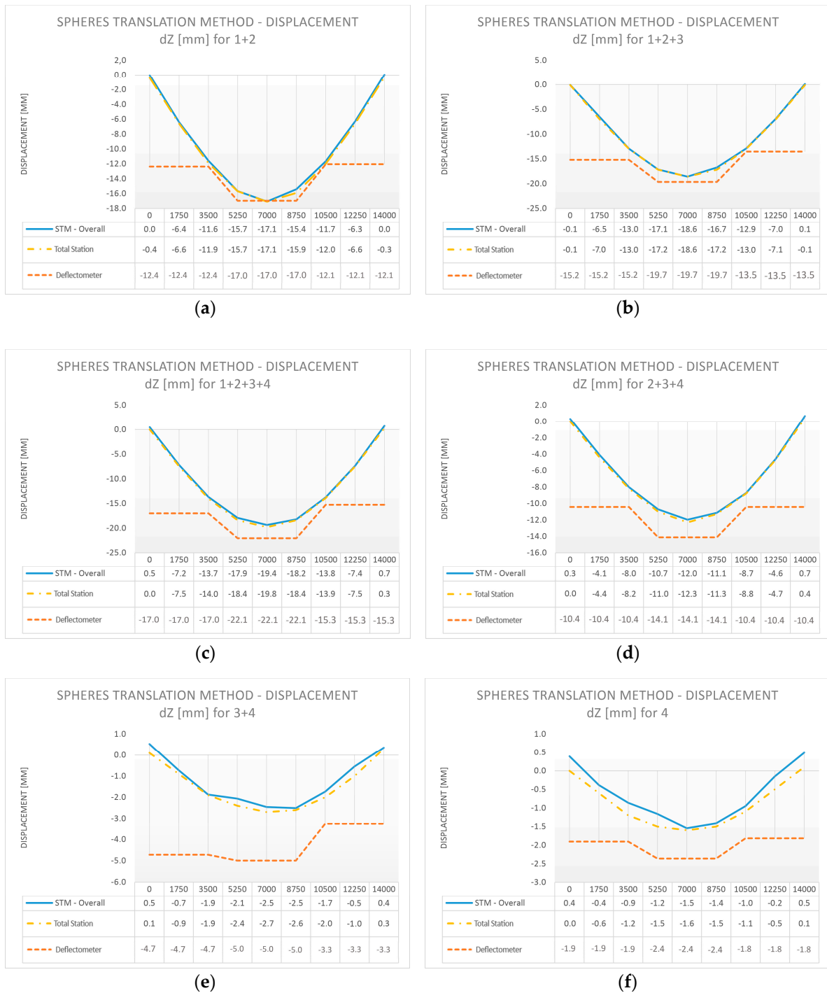
Figure 14. Displacement of the bridge diaphragm in the vertical direction during proof loading: STM in three sections + total station + deflectometer [mm]; (a) Load U1: 1 + 2; (b) Load U1: 1 + 2 + 3; (c) Load U1: 1 + 2 + 3 + 4; (d) Load U1: 2 + 3 + 4; (e) Load U1: 3 + 4; and (f) Load U1: 4.
