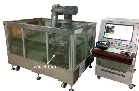
Figure 5. Overview of the robot-assisted UT system.
