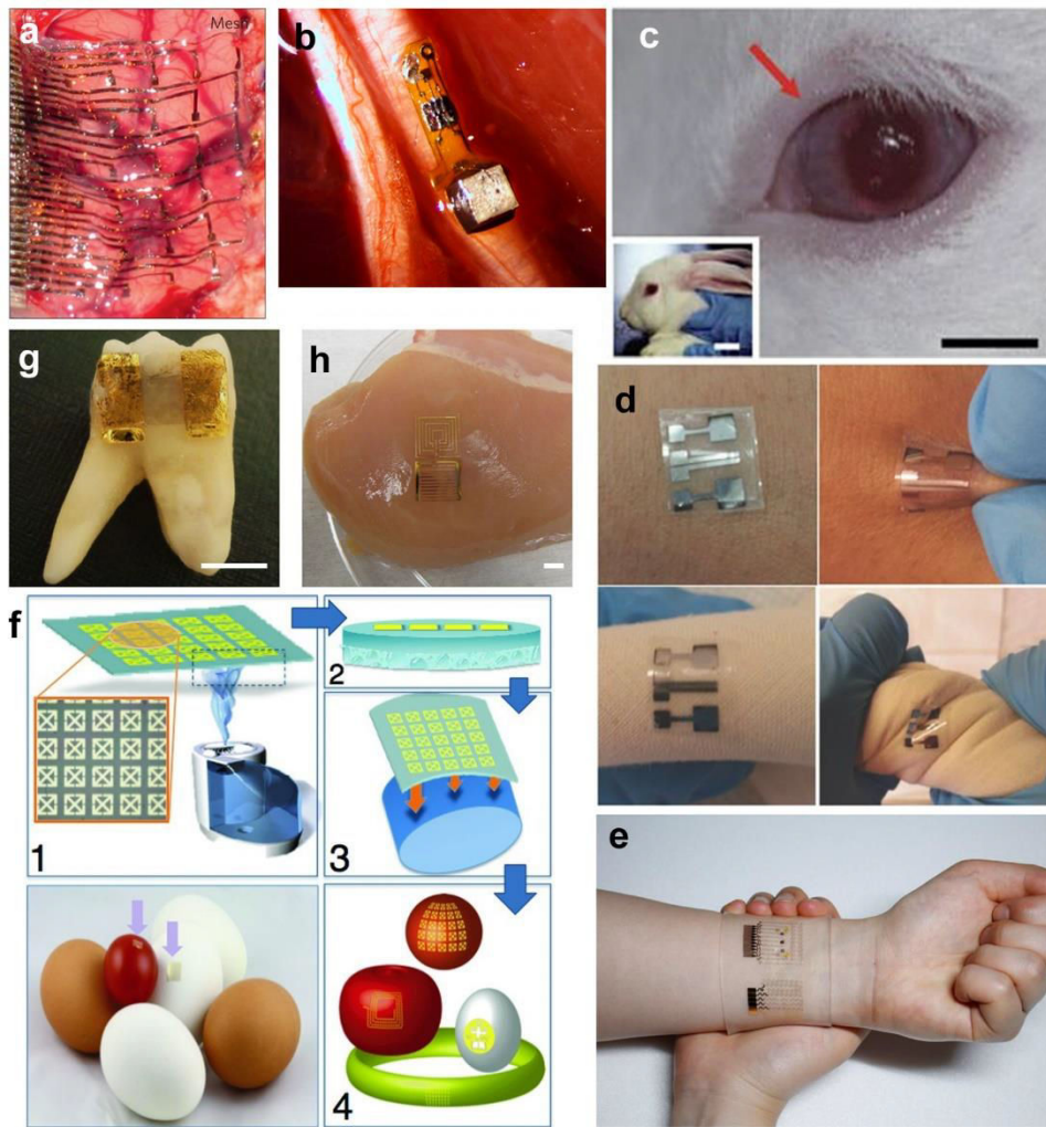
Figure 2 –. Examples of locations where flexible biosensors may be or are already being used. Clockwise from top: a) soft tissue such as the brain Adapted with permission from ref.(Kim et al. 2010). Copyright 2010 Nature Publishing Group. b) nerve fibers Adapted with permission from ref. (Seo et al. 2016). Copyright 2016 Cell Press. c) eyes/cornea (as optical implants or soft contact lenses) Adapted with permission from ref. (Kim et al. 2017). Copyright 2017 Nature Publishing Group. d, e) skin and other flexible environments, Adapted with permission from ref.(Liao et al. 2015a). Copyright 2014 Wiley. Adapted with permission from ref. (Lee et al. 2016a) Copyright 2016 Nature Publishing Group. f) surfaces of fruits and agricultural products Adapted with permission from ref. (Tao et al. 2012). Copyright 2012 Wiley. g) Enamel, h) muscle tissue. Adapted with permission from ref. (Mannoor et al. 2012). Copyright 2012 Nature Publishing Group.
