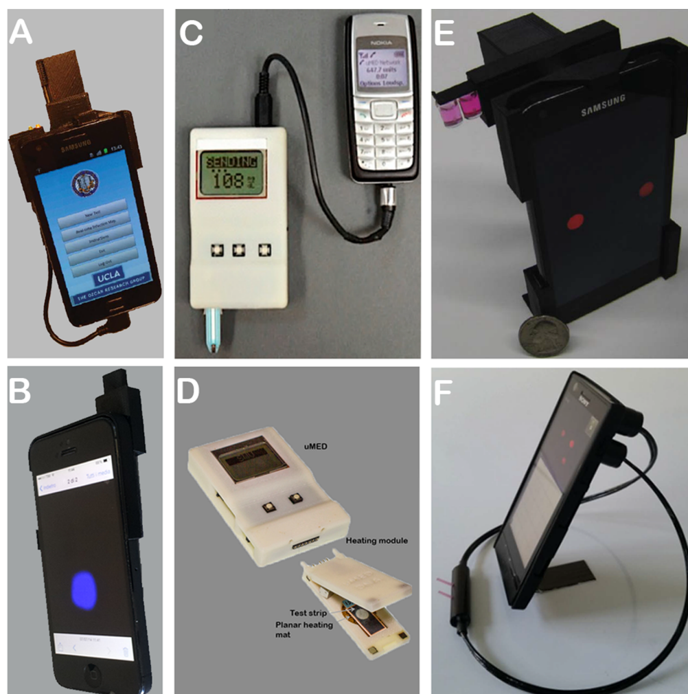
Figure 2. Examples of modified smartphones and dedicated devices for signal acquisition and data transmission to the cloud: (A) smartphone for reading lateral flow tests; (B) smartphone for bio-chemiluminescent detection on paper devices; (C) multifunctional electrochemical detector for performing various types of electrochemical techniques (e.g., chronoamperometry, pulsed voltammetry, potentiometry) using readily available electrodes; (D) updated version of device C that facilitates temperature control and electrochemical detection on paper-based devices; (E) smartphone for liquid-based colorimetric assays; and (F) surface plasma resonance biosensor installed on a smartphone. The figures were reproduced with permission from refs 111 (A), 108 (B), 180 (C), 174 (D), 179 (E), and 191 (F).
