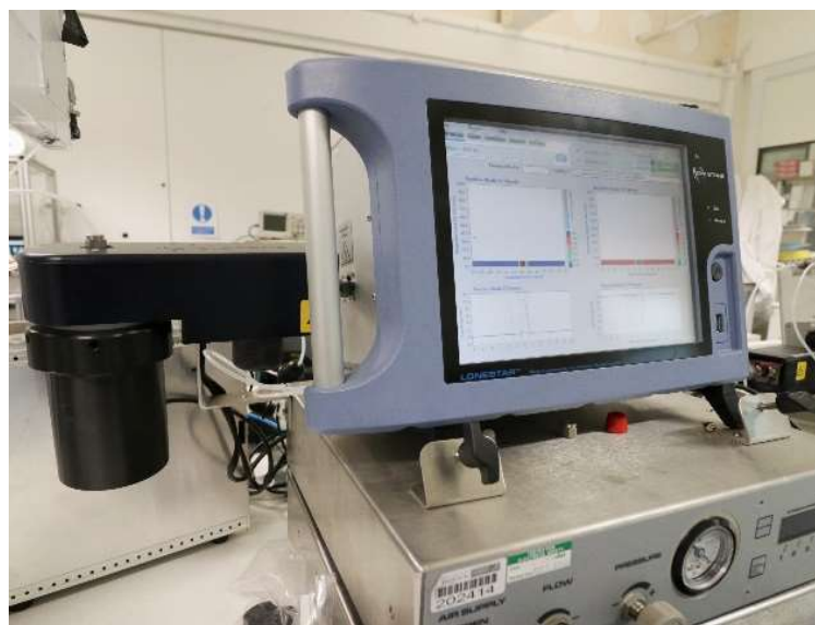
Figure 1. Field-asymmetric ion mobility spectrometer (FAIMS) setup.
