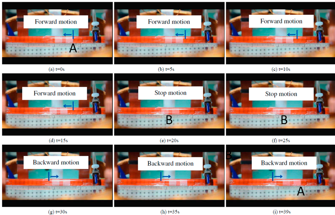
Figure 15. Forward-Stop-Backward motion. (a–d) shows the forward motion of the microrobot. (e,f) shows the microrobot stop at a point. (g–i) shows the backward motion of the microrobot.
