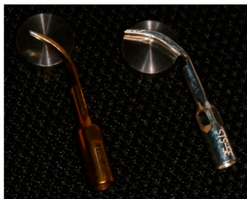
Figure 1. Photograph of conventional steel tip and copper alloy silver-plated tip on grade IV unalloyed titanium discs.
