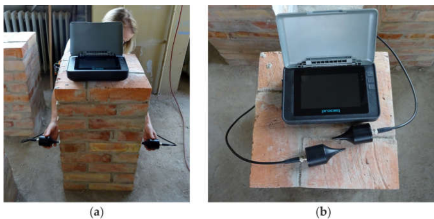
Figure 4. Experimental setup: (a) testing in through transmission mode; (b) registration unit and exponential transducers.
