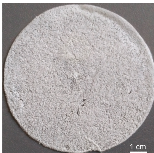
Figure 4. The porous material from butyric-acetic chitin co-polyesters 90/10 and NaCl as the porophor agent in the membrane form.
