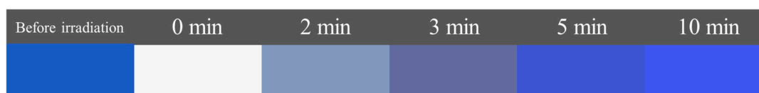
Figure 8. The color change in the oxygen indicator during recovery (in air).
