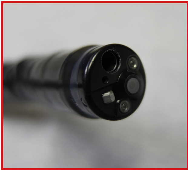
Figure 3. The tip of the endocytoscope. It has the function of a contact microscopy system with 520-fold magnification power, and it also works as an ordinary high-definition colonoscope.
