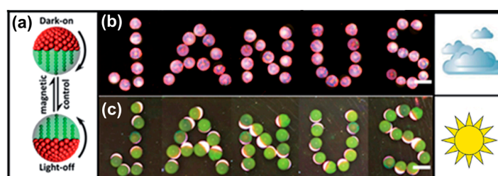
Figure 16. Magnetic Janus supraparticles (a) switched using the different hemispheres at different light intensities: upwards directed (b) PS hemisphere at low light intensity or (c) \text{Fe}_3\text{O}_4 -TMPTA hemisphere under strong light intensity; scale bars are 500 \mu\text{m} . Adapted with permission from [117] (p. 9435). Copyright 2014 Royal Society of Chemistry.
