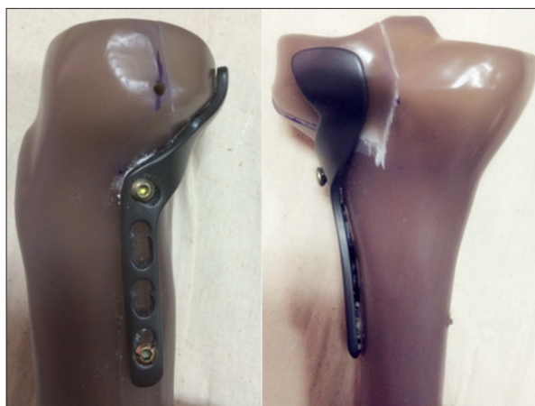
Figure 1. Diagram of the novel plate for posterolateral tibial plateau fractures in design and entity.
