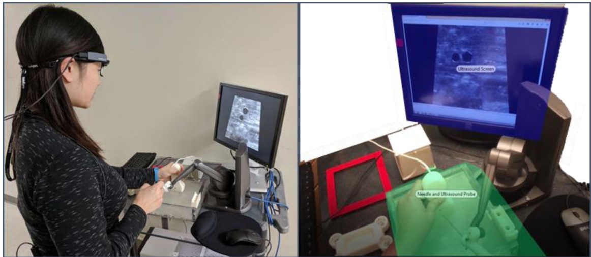
Figure 1: (Left) Experimental setup with participant wearing Tobii Pro Glasses 2 at the DHRT system. (Right) Two main areas of interest (AOIs). The ultrasound screen and the needle and ultrasound probe .
