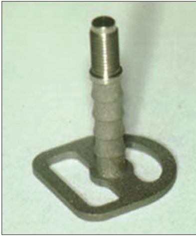
Figure 1: Single base-plate lateral basal implant with ribbed shaft and full sandblasting, as used since the mid-1990s. The surface enlargement implemented the ideas that circulated in mainstream dental implantology, where it was claimed that to obtain better retention, the surface of the implant had to be roughened
