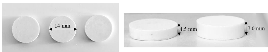
Fig. 2. (a) Appearance of freeze-dried milk/infant formula-cinnarizine tablets and (b) thickness of freeze-dried milk tablets, left = without PVPP, right = with PVPP.
