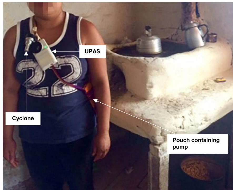
Figure 1. A participant wearing both the UPAS and the typical pump and filter gravimetric samplers. Note that both the cyclone from the pump and filter setup and the UPAS are approximately located near the participant's breathing zone.
