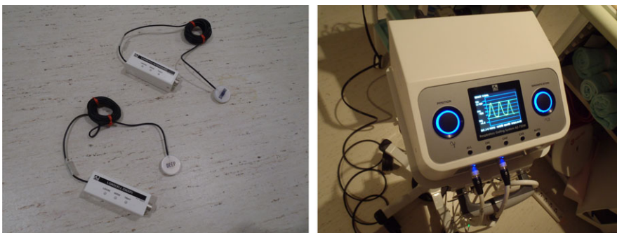
FIG. 1. Left panel: Pressure sensors (two types with different responses). Right panel: Sensor port located beside the patient couch.
