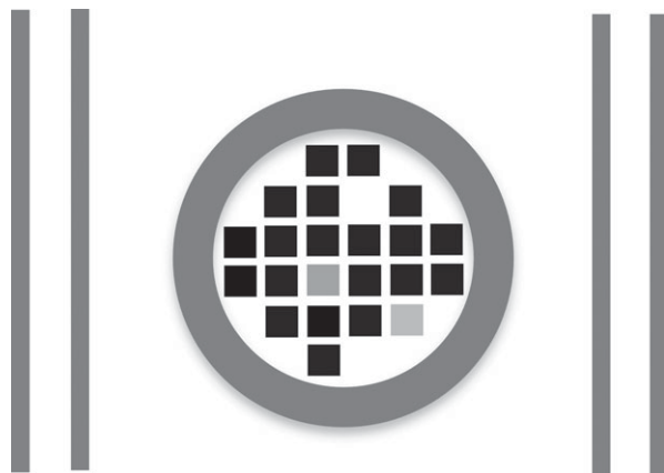
Figure 1. The layout of the detector system and a MC-10 spent fuel cask.
