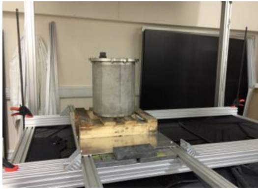
Figure 5. The Sellafield Demonstration Top Hat within the Demonstrator MIS during data collection. (Online version in colour.)
