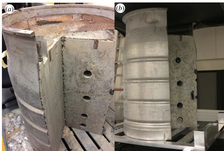
Figure 7. Photographs of the Lillyhall 500-litre ILW drum prior (a) and during (b) installation in the Demonstrator MIS. Shown are the four 60 mm-diameter horizontal cores. The two vertical cores are not pictured. (Online version in colour.)
