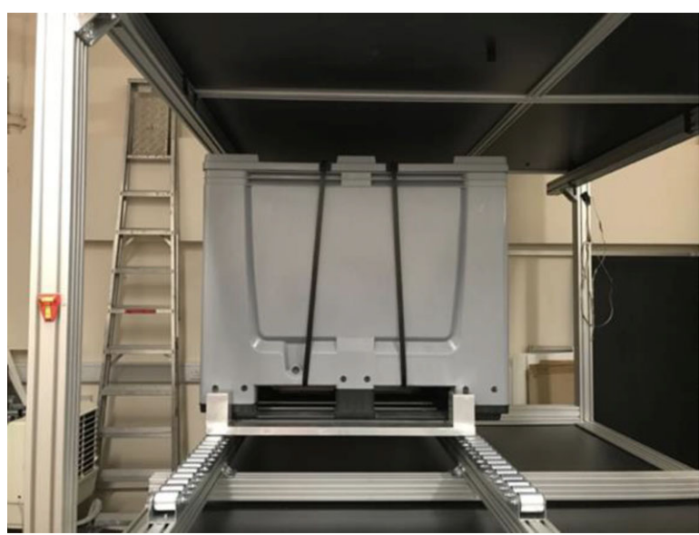
Figure 9. A GeoMelt ® sample installed in the Demonstrator MIS imaging volume inside its plastic transport box. (Online version in colour.)
