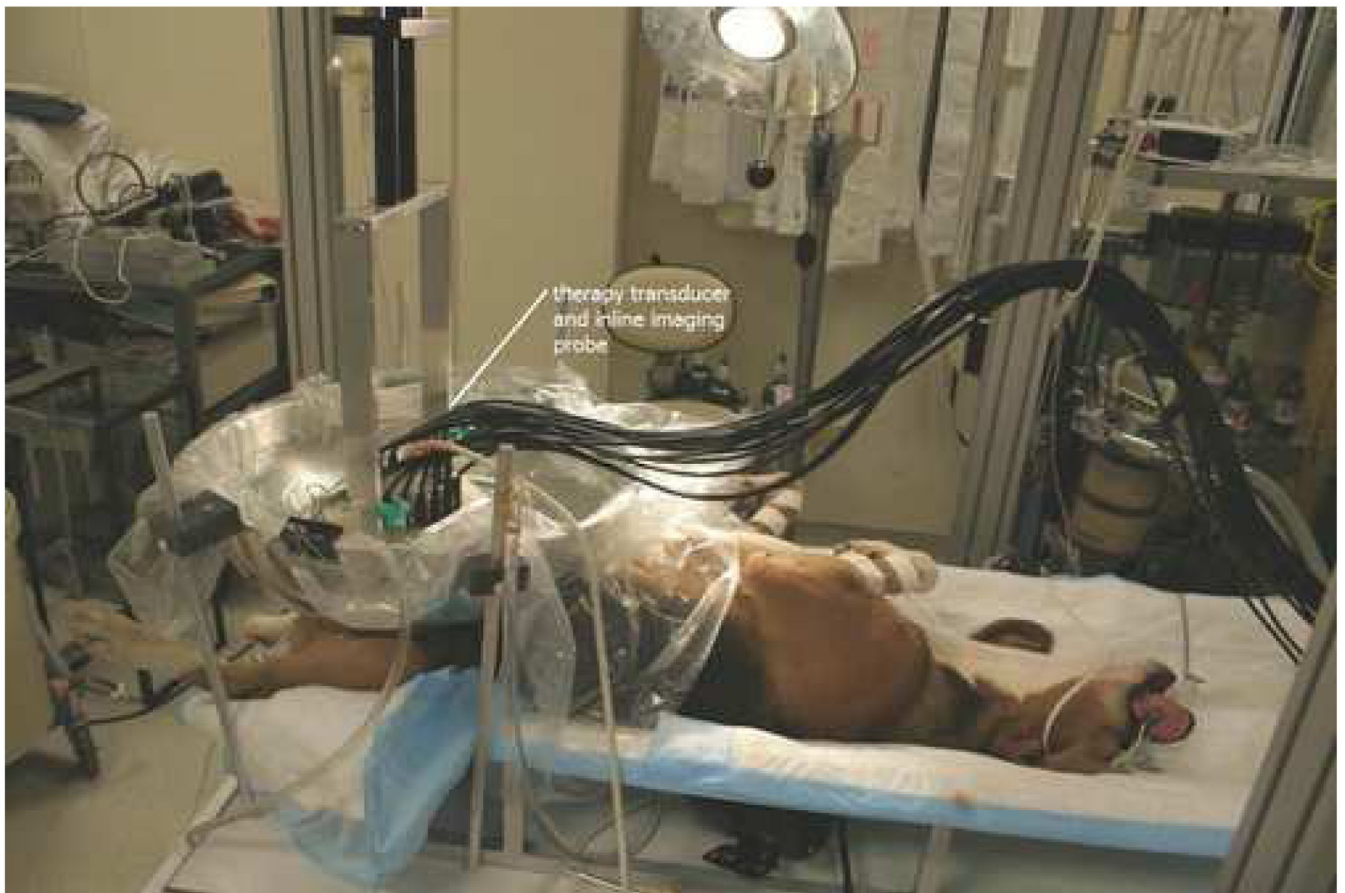
Figure 1. Picture of experimental setup. A diagnostic 5 MHz imaging probe was aligned through the center of the phased therapeutic. A circular opening in the bottom of the metal bowl was centered over the targeted zone. The bowl was lined with clear plastic and filled with degassed, de-ionized water.
