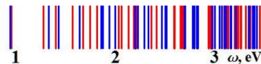
Figure 28. EM resonances spectrum for a conical resonator. The opening angle of cone is 30^\circ , the refractive index is n = 4 , and the height is h = 595 nm. The red and blue lines correspond to frequencies of electric and magnetic resonances, respectively, reprinted with permission from [18], the Optical Society (OSA).
