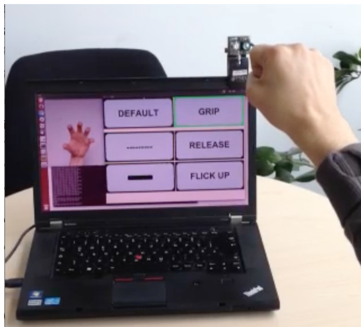
Figure 14. An exemplary hand gesture recognition setup. A user performs a dynamic gesture defined by a starting pose and an ending pose. For a dynamic grabbing gesture, pose class s_i^{start} = h (grab) starts the sequence which s_{i+m}^{end} = f (fist) ends. See Figure 6 for an overview of our ten hand pose classes. Our machine learning systems recognise the individual poses and an algorithm on top tries to identify the sequence.
