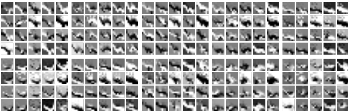
Figure 16. Resulting filter activations for the 20 kernels in the first layer of our CNN model from Figure 15. This figure shows the filtered activation for each hand gesture, grouped as in Figure 6.
