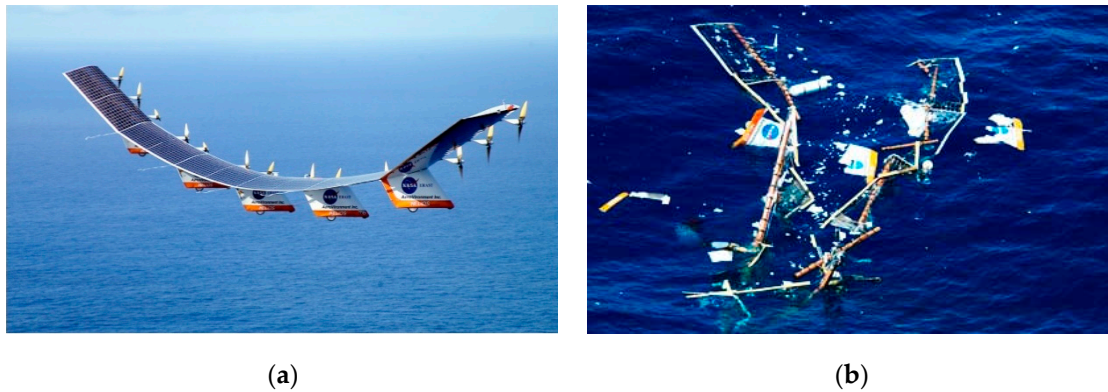
Figure 1. (a) Test photos of Helios Solar powered UAV; (b) Aerial disintegration photos of Helios [1–3].
