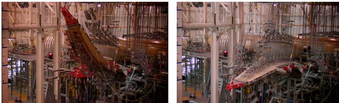
Figure 12. Detection of structural deformation through strain gages.
