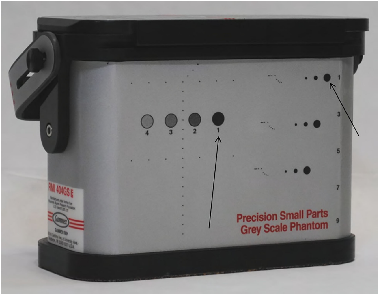
Figure 1. Gammex small parts grey scale phantom used in image acquisition. Arrows point to the two cystic structures imaged as the simulated near zone (cystic target) and far zone (grayscale target) vessels. Ultrasound images obtained from these vessels are shown in Figure 2.
