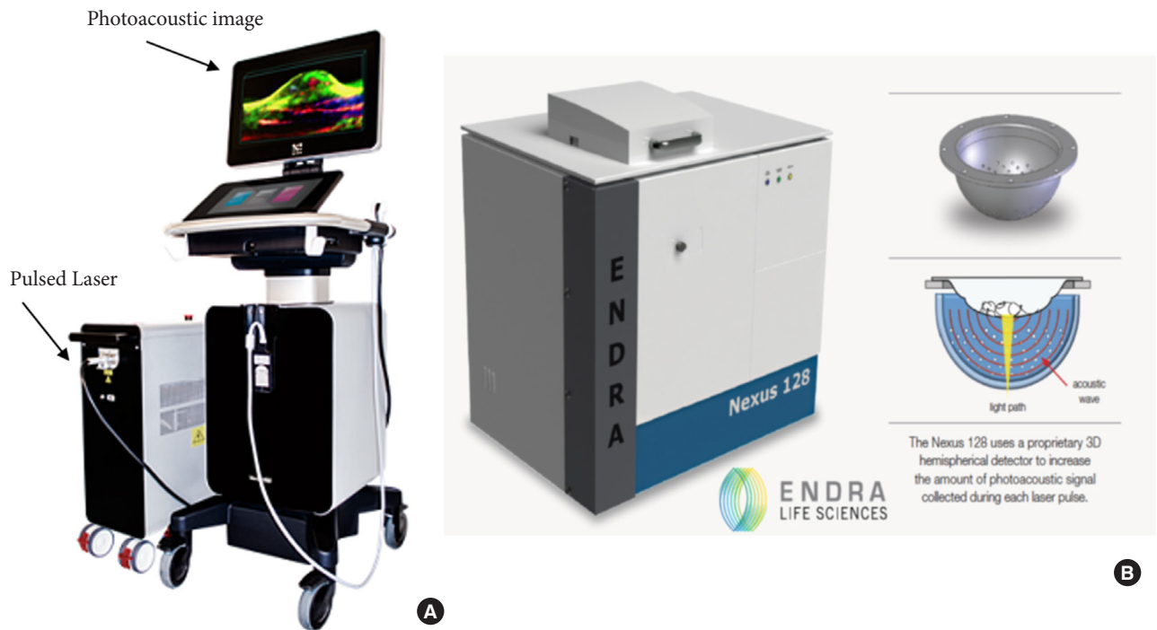
Fig. 5. Two commercially available preclinical photoacoustic imaging systems. (A) The Vevo LAZR-X (VisualSonics, Toronto, ON, Canada) uses intersecting planar laser beams (laser: 680–970 nm and 1,200–2,000 nm). (B) The Nexus 128 (Endra Life Sciences, Ann Arbor, MI, USA) delivers diffuse laser light and detects ultrasound waves using 128 transducers in a helical arrangement for 3-dimensional reconstruction.
