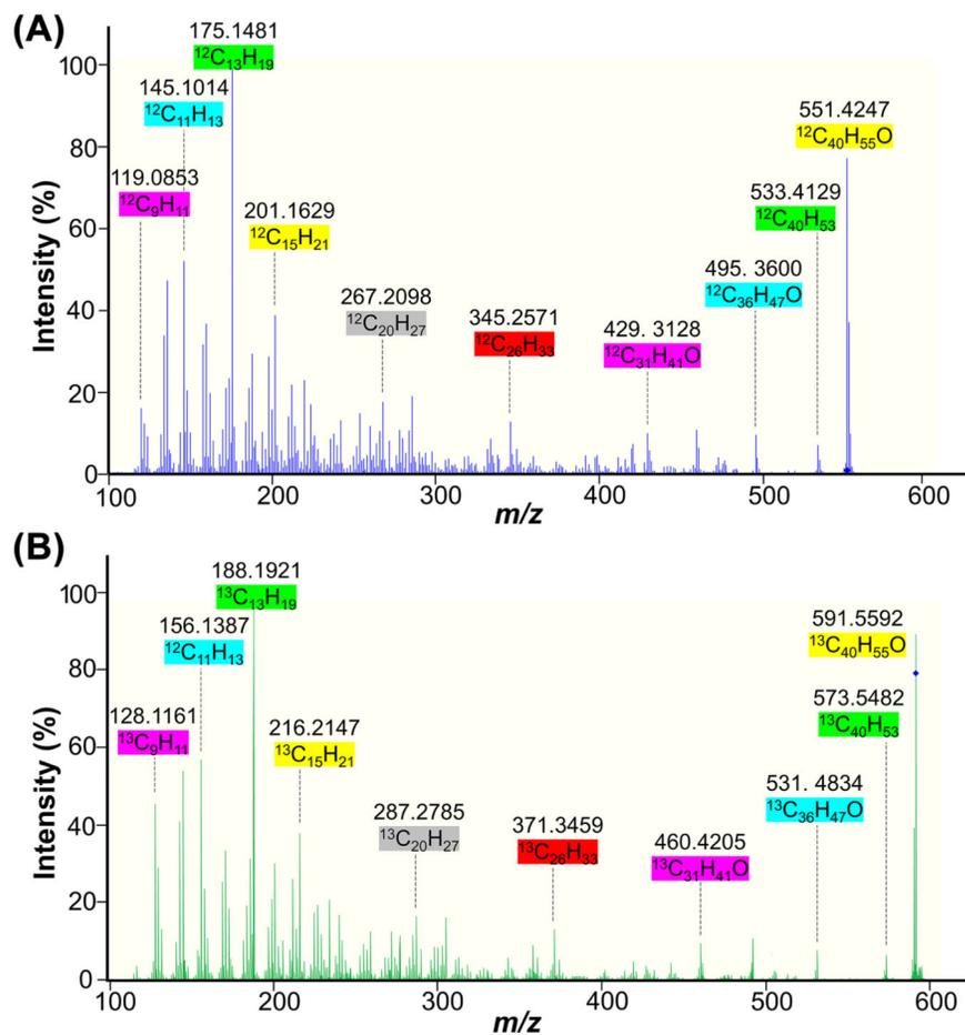
**Fig. 3.** Tandem mass spectra of the fragmentation of unlabeled standard of  $^{12}\text{C}$ -lutein ( $^{12}\text{C}_{40}\text{H}_{56}\text{O}-\text{H}_2\text{O}$ ;  $m/z$  551.4247) (A), and the  $^{13}\text{C}$ -lutein- $\text{H}_2\text{O}$  ion ( $m/z$  591.5592) from the dosed monkey liver extract (B).
