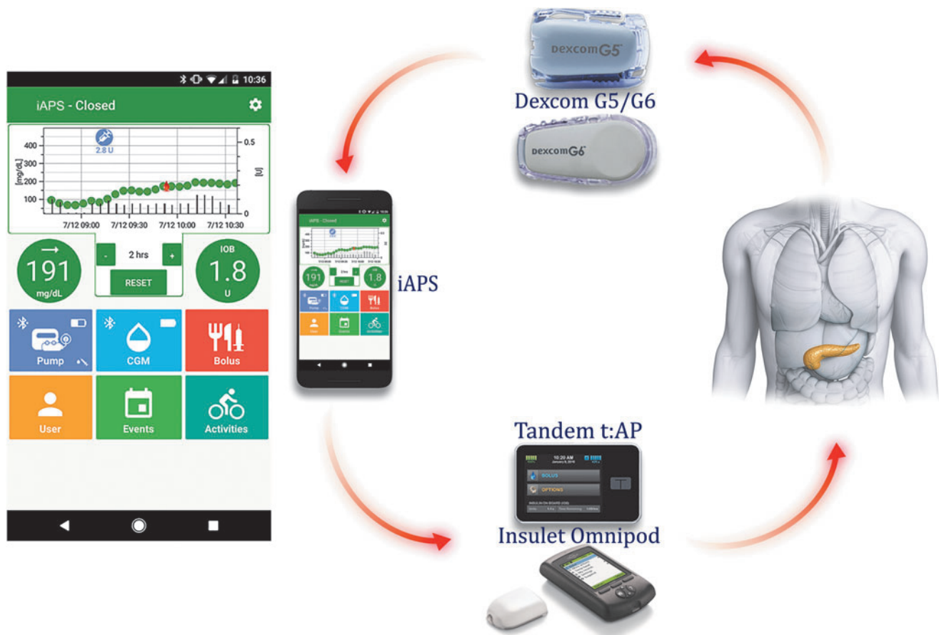
FIG. 1. Overview of the iAPS system components: smartphone running the client app, Dexcom G5/G6 CGM, and Tandem or Insulet insulin pumps. The app main screen provides access to pump, CGM, bolus, user, event, and activity pages along with graphical display of glucose and insulin history, current CGM and its trend, and IOB values. CGM, continuous glucose monitor; iAPS, interoperable artificial pancreas system; IOB, insulin-on-board.
