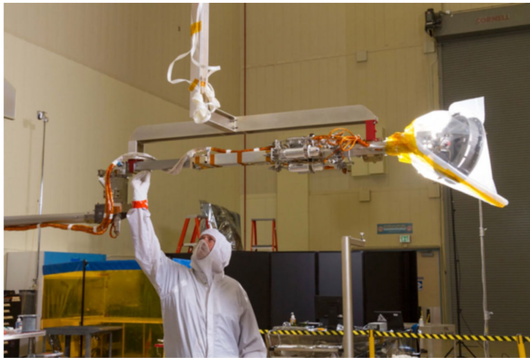
Fig. 4. Personnel properly gowned in the LM ISO 7 cleanroom and TAGSAM head protected by a PFTE bag
