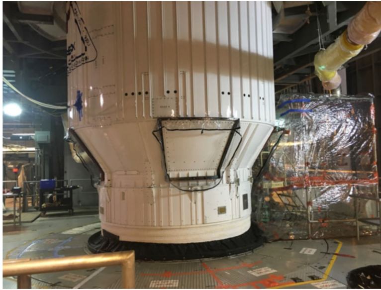
Fig. 26. OSIRIS-REx fairing “boat tail” doors and one clean tent are nearly ready to be removed for final closeout
