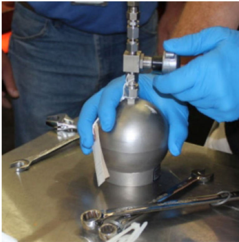
Fig. 16. Gas sampling was performed using 500-mL evacuated containers. This collection is of the purge system for the truck transport of the fairing-encapsulated spacecraft from the PHSF to the launch complex
