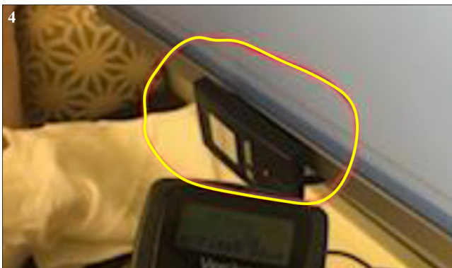
Fig. 4 Showing the RF card (WaveID) card reader in the patient room that transmits at 125 kHz. Official permission was obtained to use Vercise brand name
