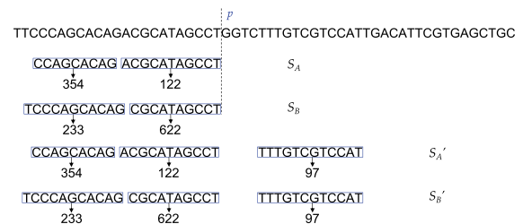
Fig. 3. Example showing that a seed subset ( S_B ) that leads to a higher frequency than another subset ( S_A ) that ends at the same location ( p ) in the read must not be part of the optimal seed solution. In this figure, the total seed frequency of S_A is smaller than S_B . Both combinations can be extended by adding a third seed, making them S'_A and S'_B respectively. For any third seed, the total seed frequency of S'_B must be greater than S'_A . Hence, S_B must not be part of any optimal solution
