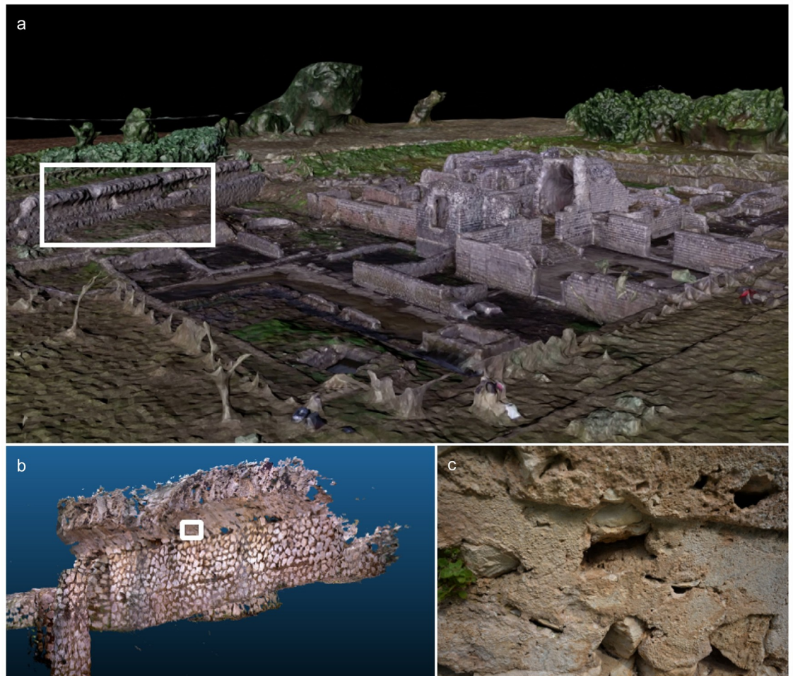
Fig 1. Collection location of the ancient Roman concrete samples used in this study. (a) 3D reconstruction of the Privernum archaeological site, collected using drone photogrammetry, (b) 3D reconstruction of the wall from which the concrete sample was collected, using a DotProduct DPI-8 3D scanner, and (c) a higher magnification photograph of the wall surface.
