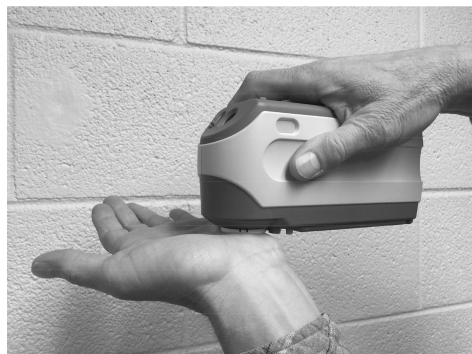
Fig. 2. Portable optical devices used for skin chromophore measurements. (a) reflection spectroscopy device and typical reflection spectrum in 400–750 nm wavelength range (Veggie Meter®, Longevity Link Corp.); (b) resonance Raman spectroscopy device and typical Raman spectrum in 900–1750 cm -1 range; (c) device based on diffuse reflection with integrating sphere (Model CM2500d, Konica Minolta, Inc.) with display of melanin and Hb indices.
