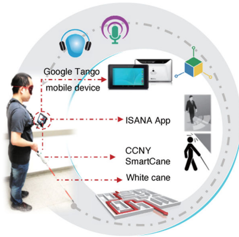
Fig. 2. ISANA and SmartCane system configuration on a blindfolded sighted subject
