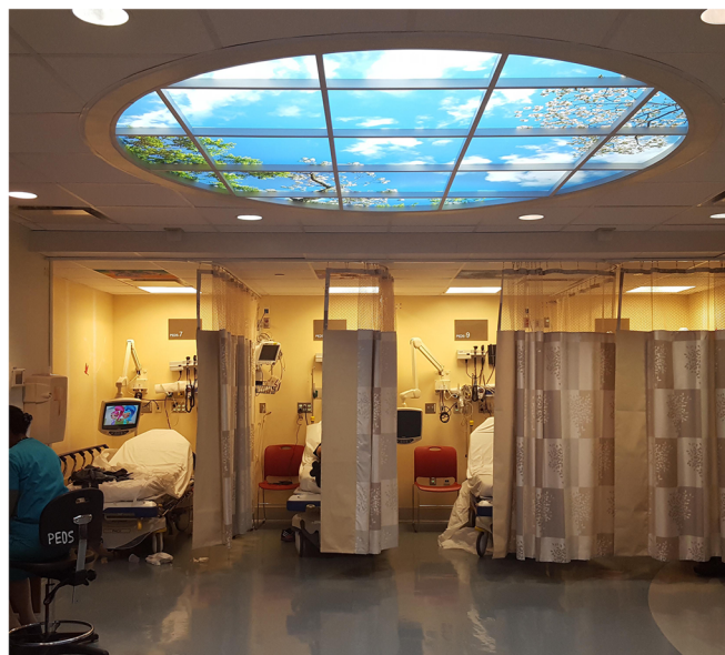
Figure 3 The Mount Sinai Health System emergency department, New York City, demonstrates an example of a virtual ceiling as a solution to existing windowless spaces (Image credit: Diana Anderson, MD, ACHA).
