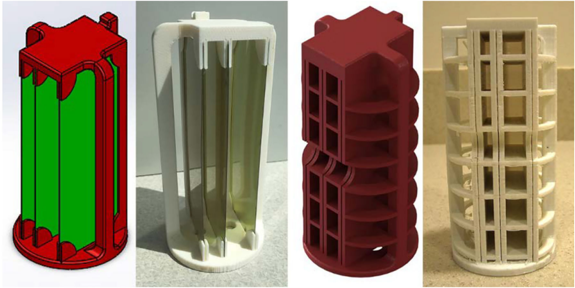
Fig 18: CAD renders and printed prototypes of iterations of coronal-sagittal film holder, version 5. The outer diameter and length of the holder are 5.7 cm and 11.7 cm, respectively. The film is 4.44 cm × 10.16 cm.
