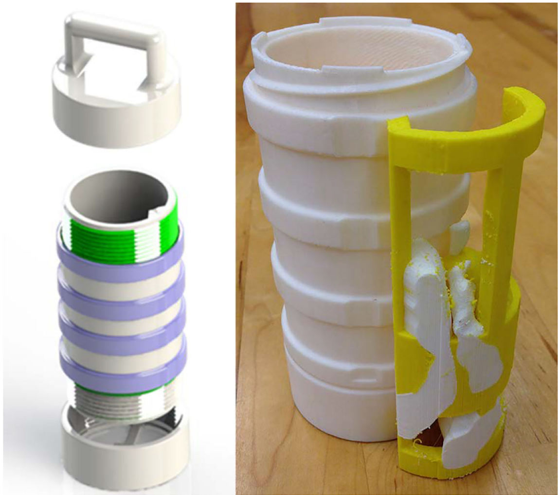
Fig 9. CAD render (left) and printed prototype (right) of the pelvis-base cartridge, version 3. The outer diameter and length of the insert are 5.1 cm and 11.75 cm, respectively.
