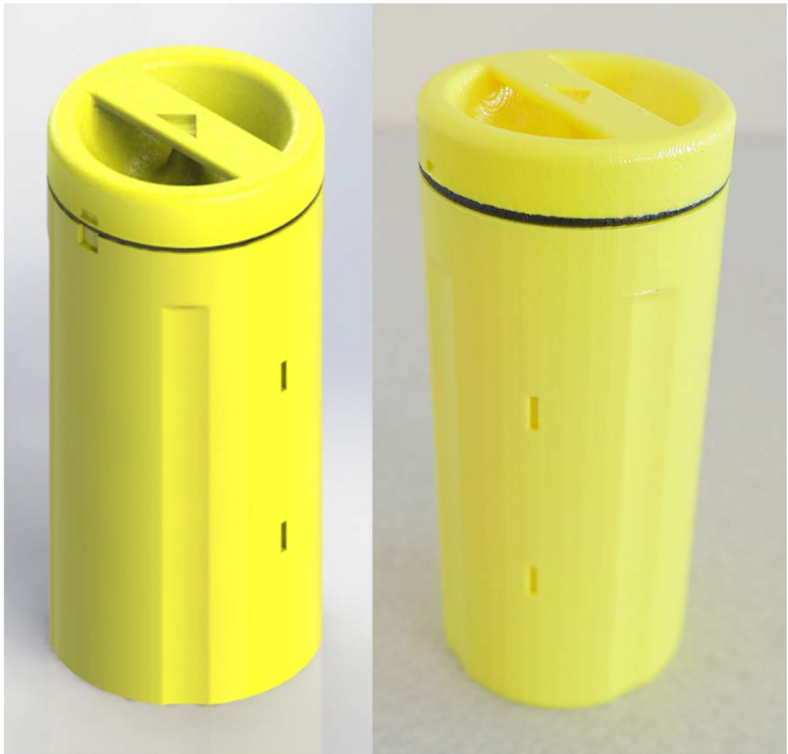
Fig 15. CAD image (left) and printed prototype (right) of the universal canister, version 5. The outer diameter, wall thickness, and length of the canister body are 6.45 cm, 0.375 cm, and 12.85 cm, respectively. It weighs 106.8 g (100% infill) and takes 7 hours and 45 min to print (alone) on a MakerBot 2×.
