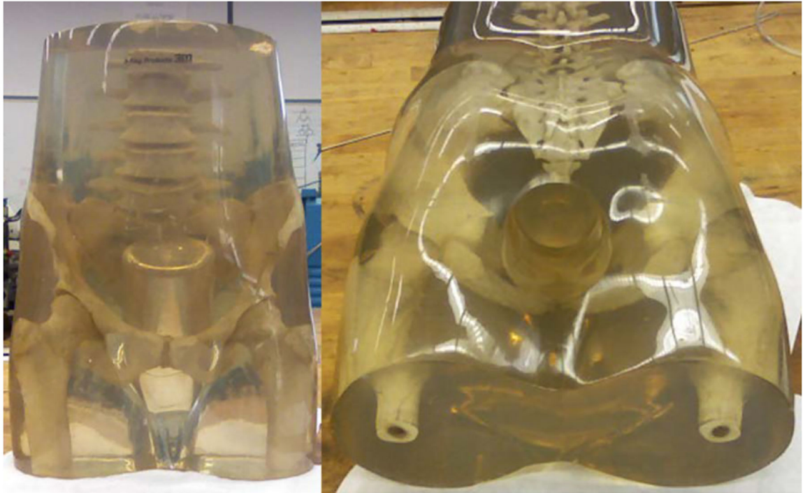
Fig. 3. Anthropomorphic pelvis base with cylindrical passage drilled out for the pelvis-base cartridge. The radiodensity of the clear, thermoplastic acrylic is equivalent to that of soft tissue.
