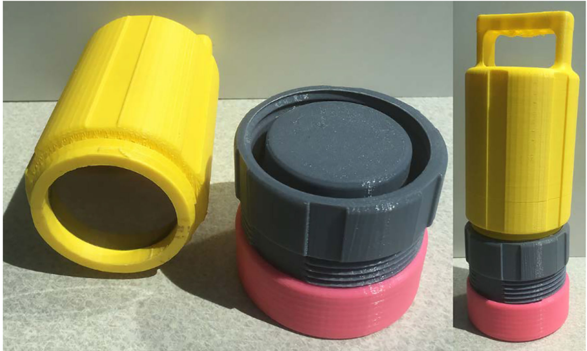
Fig. 5. Printed prototype of pelvis-base cartridge, version 1, axial orientation. The outer diameter and length of the main body (yellow) are 6.35 cm and 15.87 cm, respectively. The length of the adjustable end cap (black and pink) as shown is 8.25 cm.
