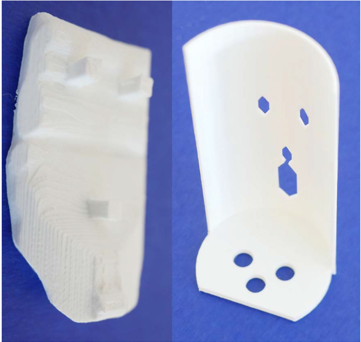
Fig. 23. Final iteration of the support frame (right). Posterior view of rectal wall part with the three square mounting pegs (left).
