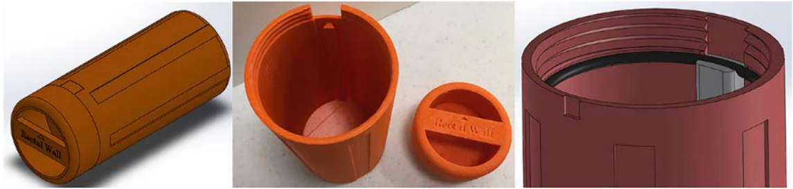
Fig. 11. CAD images (left, right) and printed prototype (center) of the universal canister, version 4. The O-ring (black, right) is only supported at one location by the backbone of the film holder (gray).
