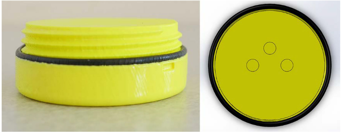
Fig 16. Printed prototype of the universal canister cap, version 5 with O-ring (left). The height of the cap is 2.5 cm. It weighs 66.3 g (100% infill) and takes 4 hrs 27 min to print (alone) on a MakerBot 2x. CAD image of the bottom of the canister showing the three alignment pegs (right).
