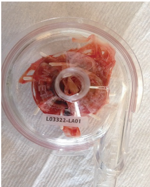
Figure 1 Oxygenator clot formation 1.
