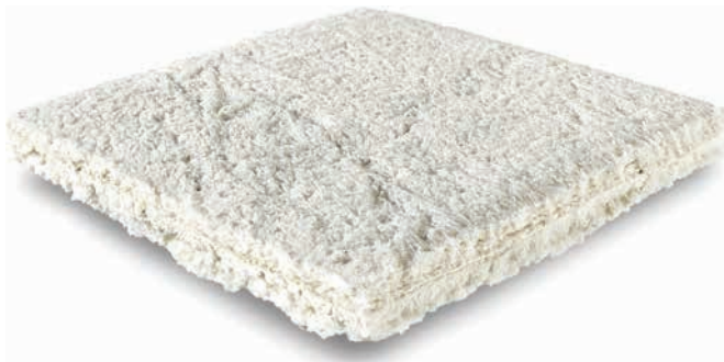
Fig. 2 - The newly developed magnesium-doped hydroxyapatite/type I collagen (MHA/Coll) 3D scaffold developed for bone regeneration.
