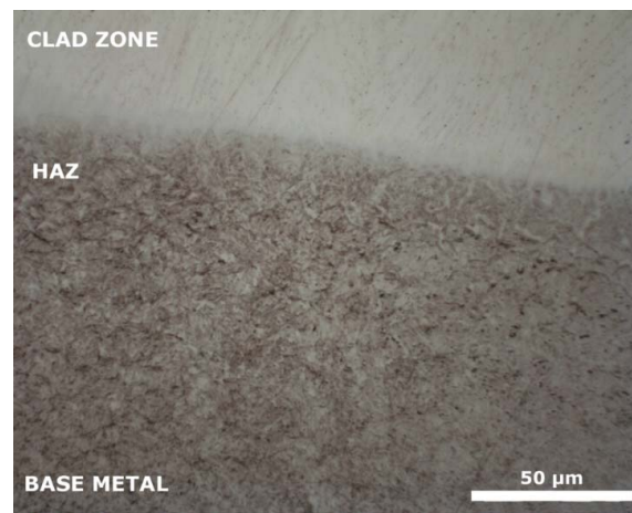
Figure 3. Detail of the three regions of interest in the cladding of sample A (10% H13).
